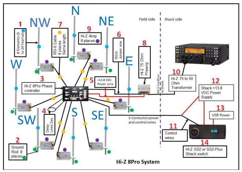
Hi-Z 4 Element Receiving System V2 Block Diagram
