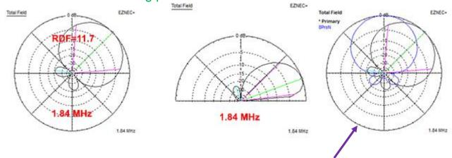
Two direction Overlap in above plot shows near 100% coverage in all directions.
