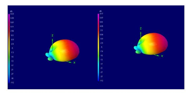
85 foot diameter 60,30 degree delay cables 113 foot diameter 80,40 degree delay cables Very similar patterns at 160 Meters with 85 or 113 foot diameter array dimension.
