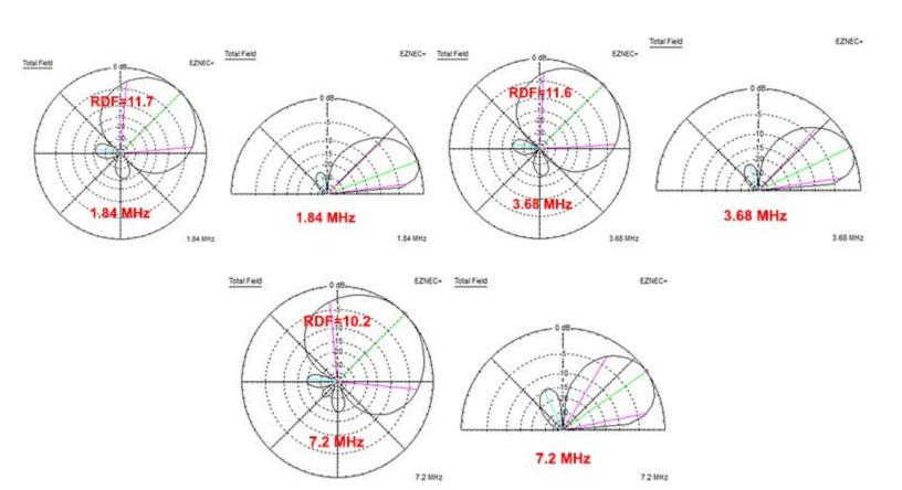
85 Foot Diameter. One customer adjusted pair of delay cables of 70 degrees for the long delay cable and 35 degrees for the short delay cable at 1.84 MHz (Max Front to Back mode) with customer modified delay cables.
