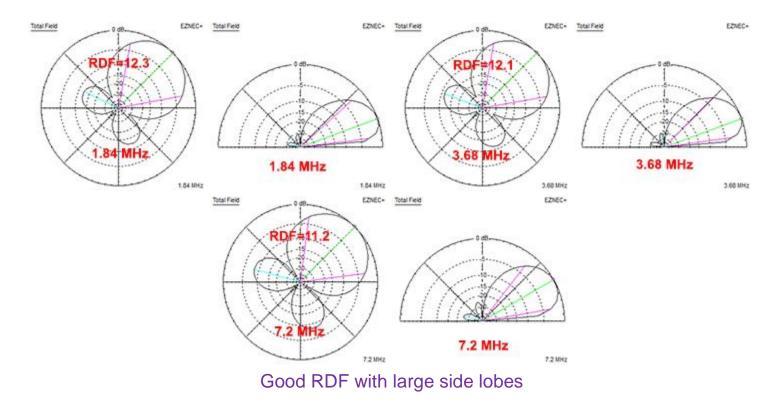
113 Foot Diameter. One pair of delay cables of 80 degrees for the long delay cable and 40 degrees for the short delay cable at 1.84 MHz
