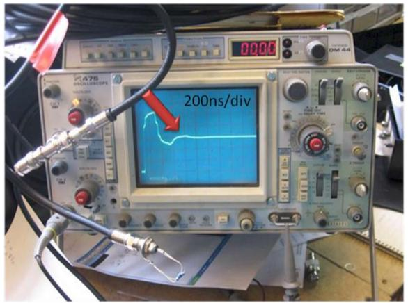
The scope time base was lengthened out in time so one can see that the reflections eventually die out after being absorbed by the load and source impedances. The time base is 200 nanoseconds per division in this picture.
