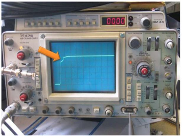
The 50 ohm terminator was replaced with a 75 ohm termination and the wiggle is a bit worse. This wiggle is fairly insignificant as any cable connected for a test, will be considerably longer and the reflections will show later in the trace. Scope settings
