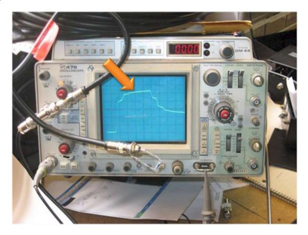
A pair of 75 ohm resistors were added in parallel as a termination on the cable. This of course terminates the cable in 37.5 ohms which shows a severe mismatch compared to the cable terminated with the 75 ohm proper termination.
