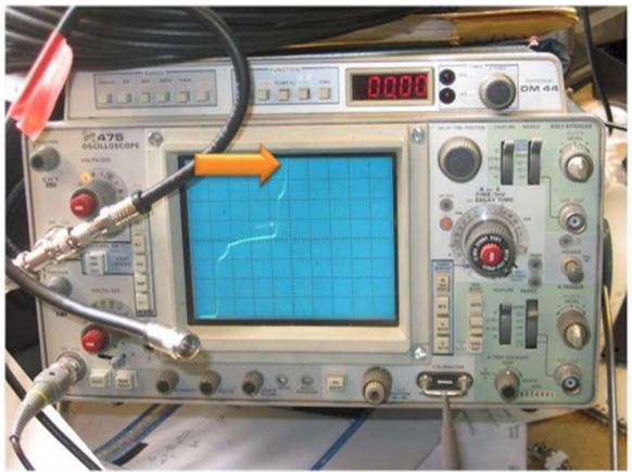
A piece of 75-ohm cable was added to the connection with no termination resistance. It is very easy to see the reflected signal coming back from the open end so large it is off scale to the top.
