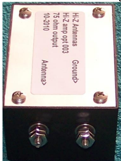
Terminals to Ground and Vertical
