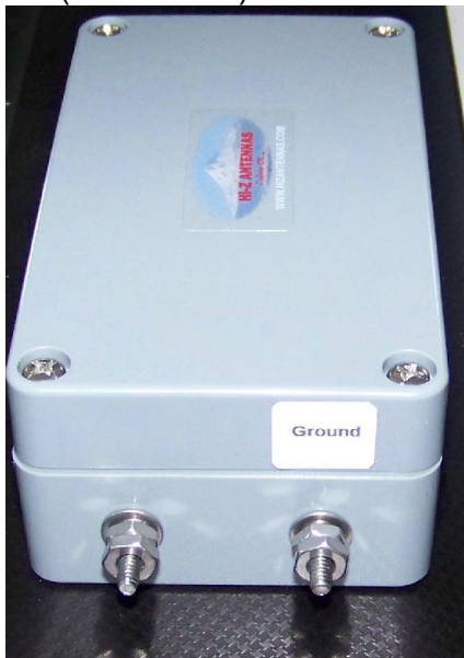
Terminals to Ground and Vertical
