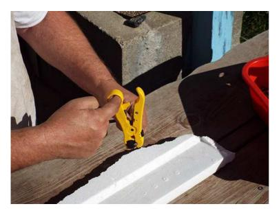
Twirl the tool several rotations until it turns easily and begins to slide off the end with a gentle tug. Do not let your finger slip out of the loop into the blade!
