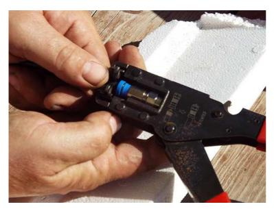
Push the connector firmly into the tool.
