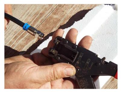
With the compression tool open as shown prepare to insert the cable.
