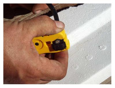
Clamp down the tool with fingers as shown to break through the insulation.
