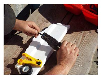
Squeeze the handles firmly which will snap and release the ratcheting handle.
