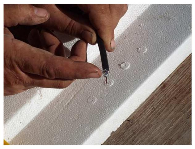
Fold back the braid only onto the outside insulation.
