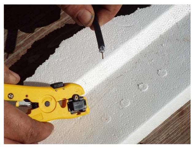
Pull the tool away exposing the trimmed cable end.
