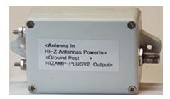
The front view size is 2 1/4 X 4 1/2 inches including mounting ears and input and output connectors. Depth is 1 3/8 inches
