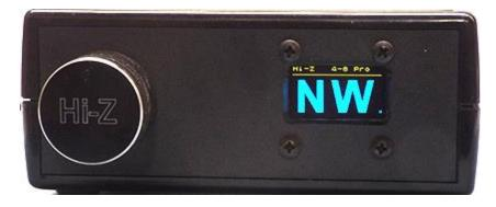
Selection of the 2 versions of Hi-Z amps available will depend somewhat on the users location. If the user is in a VERY quiet RF location on the lower bands then the HIZ-AMP-PLUS is reccommended. Using the HIZ-AMP-PLUS may also preclude the need for an array post amplifier if 20 to 24 foot elements are used. Using thin diameter or wire 15 to 20 foot elements or less in normal quiet suburban areas one should use the HIZ-AMP-PLUS which has 6 dB more gain and lower noise figure.
