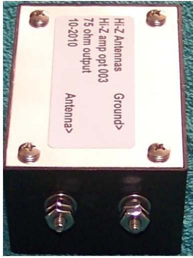
Terminals to Ground and Vertical
