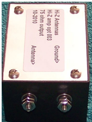
Terminals to Ground and Vertical
