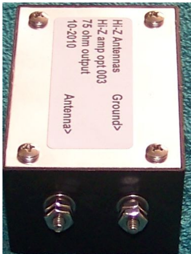
Terminals to Ground and Vertical
