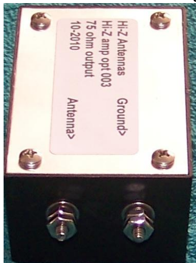
Terminals to Ground and Vertical
