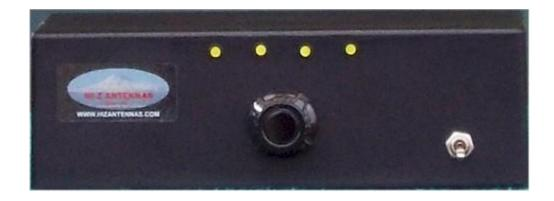
Simple front panel controls include a power on and off switch plus selector rotary switch. Led lights indicate the selected direction. Personalized labels can be used for information. One of the LEDs will always be on as an indicator when the power is switched on.
