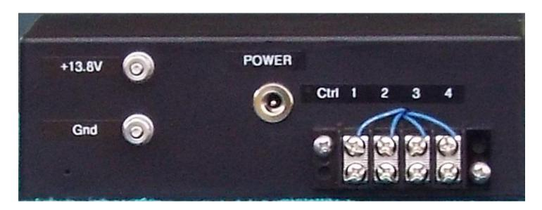
Rear panel connections are pretty straight forward with input 1 being the front panel switches most counter clock wise position and the left most LED is on. Input number 4 is for the most clockwise position and last LED is on. The others follow suit in order. Customer supplies the cable to the remote switch.
