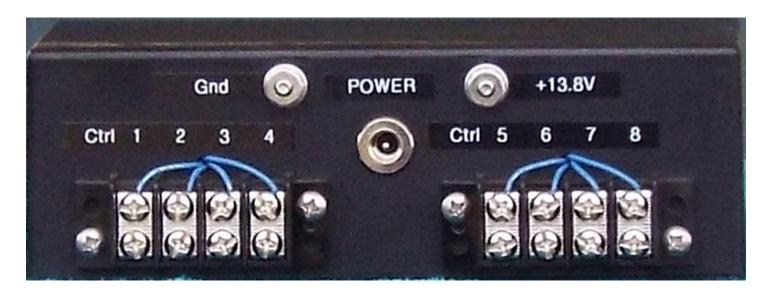
Rear panel connections are pretty straight forward with input 1 being the front panel switches most counter clock wise position and the left most LED is on. Input number 8 is for the most clockwise position and last LED is on. The others follow suit in order. Customer supplies the cable to the remote switch.
