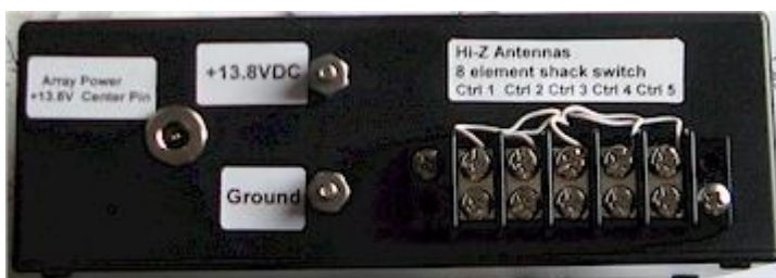
Rear View – Shack Switch
