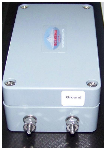
Terminals to Ground and Vertical
