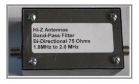
This 75-ohm band-pass filter is designed to provide receiving array protection from local high-powered A.M. broadcast stations. This filter is fitted with 75-ohm type F connectors and will provide out of band attenuation as seen in the chart below. Insertion loss is an average 2 dB in the pass band. Attenuation is a 35 dB at 1600 KHz and as can be seen, much more at lower frequencies. The band pass 3-dB corners are at 1.8 MHZ and 2.0 MHz.
