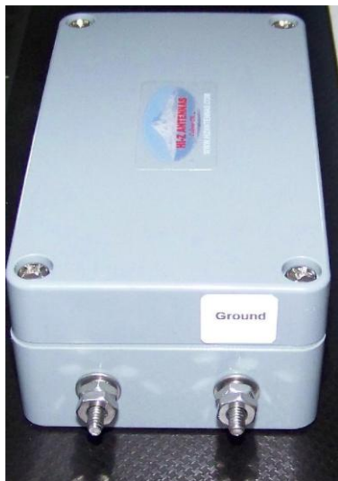
Terminals to Ground and Vertical
