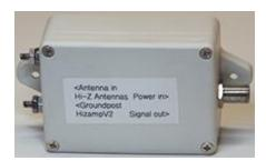
The front view size is 2 1/4 X 4 1/2 inches including mounting ears and input and output connectors. Depth is 1 3/8 inches
