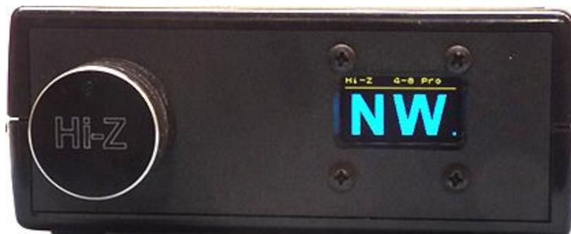
Selection of the 2 versions of Hi-Z amps available will depend somewhat on the users location. If the user is in a VERY quiet RF location on the lower bands then the HIZ-AMP-PLUS is recommended. Using the HIZ-AMP-PLUS may also preclude the need for an array post amplifier if 20 to 24 foot elements are used. Using thin diameter or wire 15 to 20 foot elements or less in normal quiet suburban areas one should use the HIZ-AMP-PLUS which has 6 dB more gain and lower noise figure.
