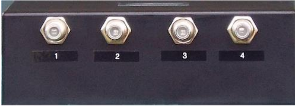
Front Panel is used to accept the 4 cables to be switched
