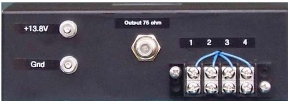
Rear panel is used for output , control, and power
